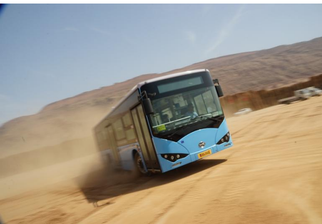
2 Months High Temperature Test (up to 48.7°C) in Turpan Summer
